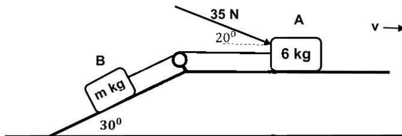
The coefficient of kinetic friction on block A is 0,2 and 0,15 for block B respectively.
