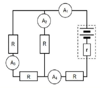
Which ONE of the ammeters in the circuit will have the LOWEST reading?
