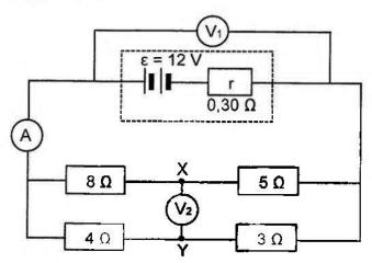
8.3 Calculate the reading on the voltmeter V2
