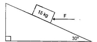
The coefficient of kinetic friction between the block and the surface is 0,20.
