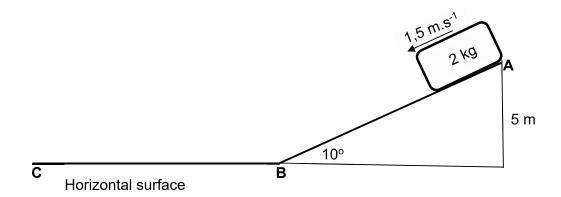
At the bottom of the plane, the object continues sliding onto the rough horizontal surface and eventually comes to a stop. The frictional force acting on the block while it slides along the inclined surface is 2,5 N.
