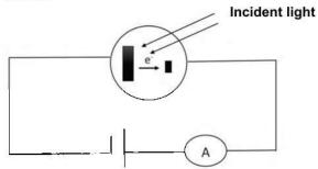
10.1 A reading is registered on the ammeter when green light is used in the photocell above.
